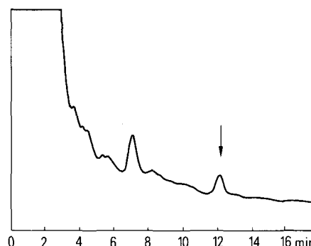
Fig. 1. Chromatogram (total ionization current of the mass spectrometer) of a purified extract of Amblyomma . A prominent peak has the same retention time (arrow) as the fully silylated derivative prepared from authentic ecdysterone (Simes, Italy). Unidentified peak at about 7 min retention time does not appear to be an ecdysteroid. Chromatographic conditions: LKB 9000 GLC-MS apparatus; column: 2 m x 2 mm OV.1 (1%) on Gas Chrom P. Temperatures: column 280°C; flash heater and separator 295°C. Flow rate of carrier gas (helium): 30 ml/min.
